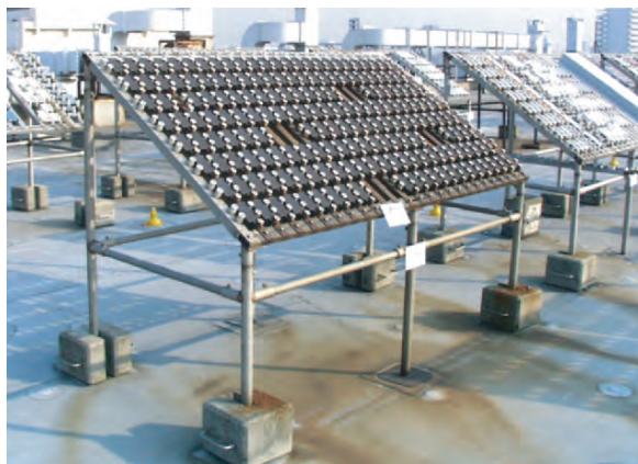
Fig. 12.4. Example of outdoor exposure test. The plates tested are insulated with ceramic insulators
