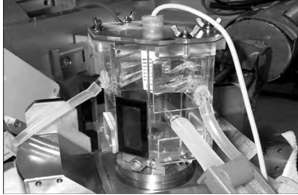
Fig. 9.10. Photograph of specially designed corrosion chamber
